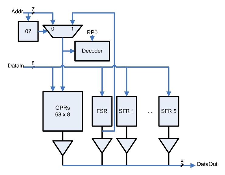
In this experiment, you need to implement address multiplexer, decoder circuit, GPRs, SFRs, and tri-state butters. The associate circuits for the SFRs should be left to Experiment 7.
